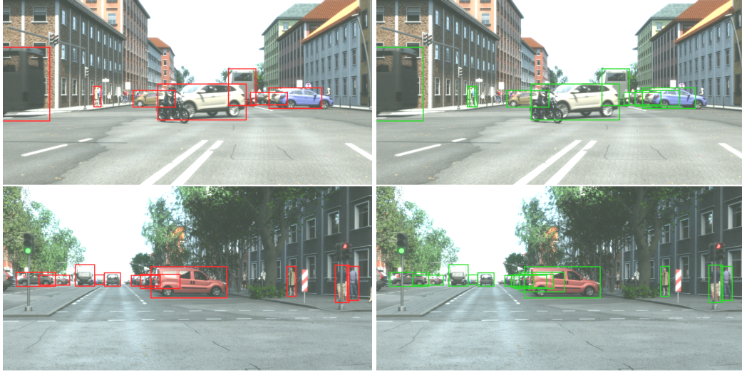
Figure 7: Left: Final detections without vg-NMS. Right: Final detections with vg-NMS.
